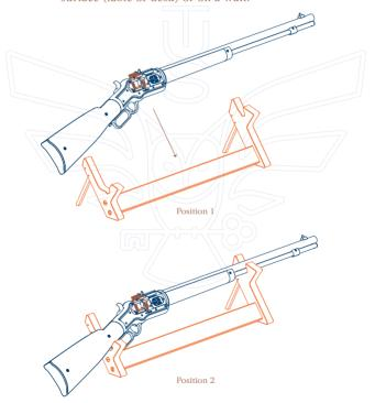
The hammer may be pulled back manually to the cocked position. To release the hammer, press the trigger. Cocking the hammer and pulling the trigger will not wind the clock.
