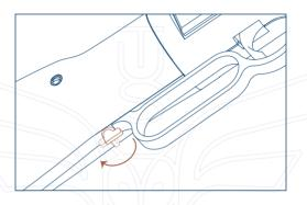
The winding mechanism replicates the action of cocking the rifle.
