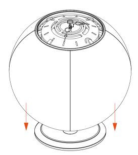
ORB's four elytra are soldered to the structure with torque hinges. If necessary, you can tighten the elytra yourself, or ask a watchmaker to make the adjustment for you.
